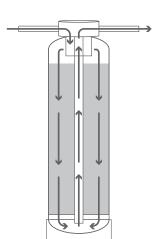
SWT's Non-Backwash Filters typically feature a composite tank with polypropylene liner, SWT's Cyclonic Distributor System (CDS), machined PVC tank head with choice of connections, and choice of filtration media. Slotted riser tubes, basket risers, hub & lateral systems, and upper screen/diffusers also available.
